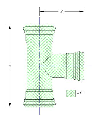
NOTE TO FABRICATORS; PLEASE WRITE ON THE FITTING THE FOLLOWING MESSAGE: GLASS TO SDR21 BETWEEN THE BELLS, 3M ON BELLS.
